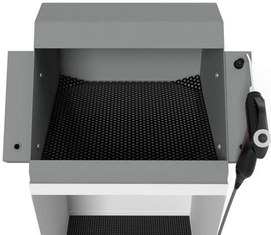
**EXOCLEAN** is equipped by a small single phase efficient electrical motor. Oilmist generated by the process of blowing parts is conveyed into the lower section of the cabin where oil is recollected into a convenient drainage tank. The mist is filtered by an M5 fiberglass cell that allows air recirculation inside the shop.
